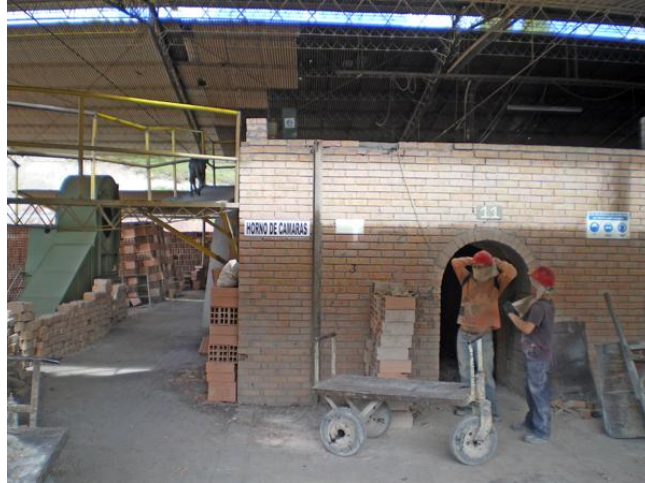
Figure 4. Chamber kiln at Santander Ceramic (project situation).
